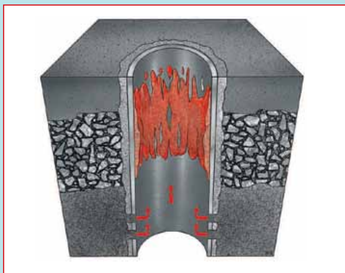
Paraffin crystals can form on tubing walls as the temperature of the produced fluid decreases
